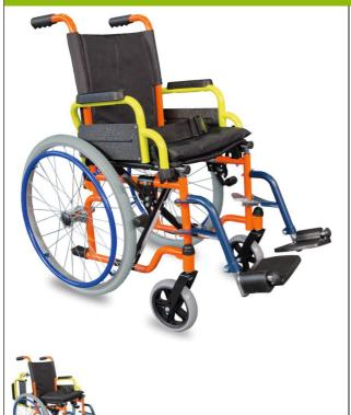
This manual wheelchair is designed for children. It folds up completely and has fold-up armrests, a fixed seat and fold-down footrests. The rear wheels are 51 cm (20') in diameter and have handrails and brakes. The front directional wheels are smaller (15 cm in diameter). An integrated belt provides better support for the user.
