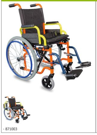
This manual wheelchair is designed for children. Folding, it features folding armrests, a fixed seat, and folding footrests. The rear wheels are 51 cm (20") in diameter and have handrails and brakes. The front wheels are smaller, with a diameter of 15 cm. A seat belt is integrated to ensure better support for the user. Steel frame.
