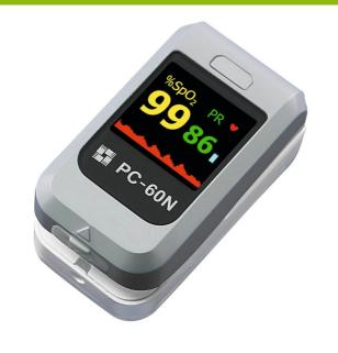
High-performance adult and paediatric finger oximeter. Can be fitted with an external clip-on or silicone paediatric sensor. Large OLED colour screen with automatic screen orientation. Adjustable visual and audible alarms for SpO2 and heart rate. Supplied with 2 LR03 batteries and 1 wrist strap. Model PC-60NW supplied instead of PC-60N.
