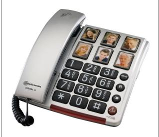
Telephone combining a large keypad with 6 programmable direct access memory keys. The listening volume is amplified up to 40 dB and the ring tone is amplified up to 90 dB. Compatible with hearing aids. Visual flash when a call is received. 10 memories.
