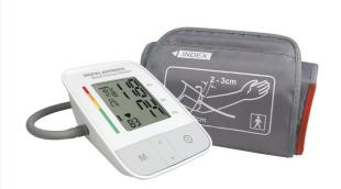
Automatic arm blood pressure monitor that silently measures the blood pressure and displays it on a large LCD screen.
