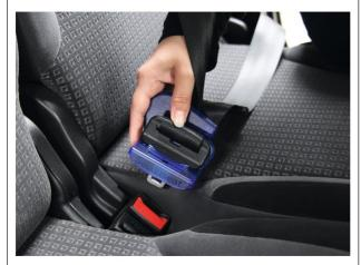
The Securiseat is a safety device for the exclusive use of disabled persons who are at risk of inappropriate behaviour during transport. Prevents seat belts from being accidentally unfastened. Once the Securiseat is locked, the seat belt cannot be removed except with the keys provided or a car key.
